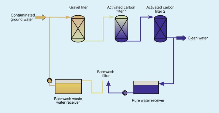
Process flowsheet for ground water decontamination applying wet activated carbon
